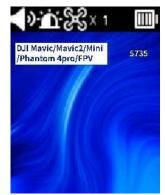
Step 4: Click on the button "Set and OK" to enter the direction finding mode, the information displayed on the direction finding mode interface from top to bottom are the drone model, drone frequency and signal strength (this value is used to determine the location of the drone).
