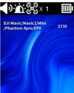
Step 3: Click on the button "Back" to select the drone that needs direction finding. When more than one drone is detected at the same time, click on the button "Up" or "Down" to select the drone to be direction-finding.
